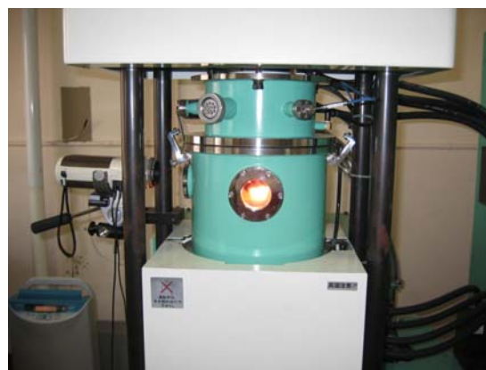
Photo. Pulse Electric Current Sintering at 1500°C
